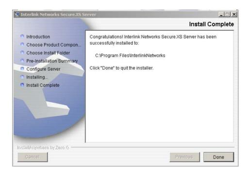
8. Test the Installation - Verify that the installation and configuration is complete and correct. This is done by running the Secure.XS Test Tool from the Start->Interlink Networks menu. Click on "Test Authentication" to start the server and send a test request. Enter the test username and password that you configured in the installation (test user, password).
